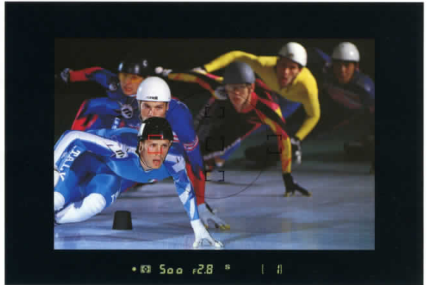
The selected focus area is superimposed on the focusing screen. The brightness of the superimposition automatically adjusts according to the degree of ambient light.
